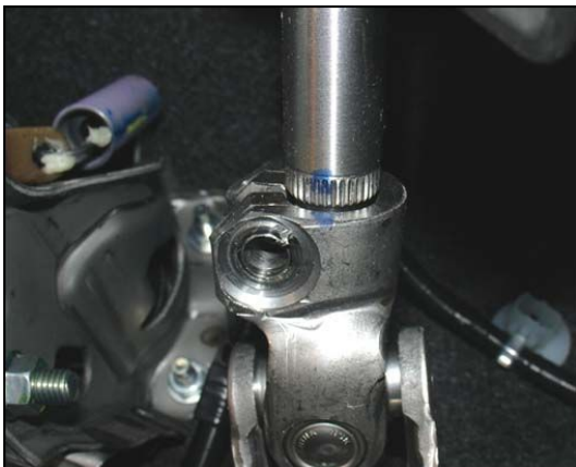
Figure 10. INCORRECT: Splines Are Showing – Not Installed Completely
