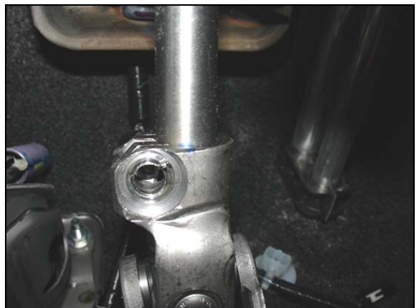
Figure 11. CORRECT: Splines Are Not Showing
