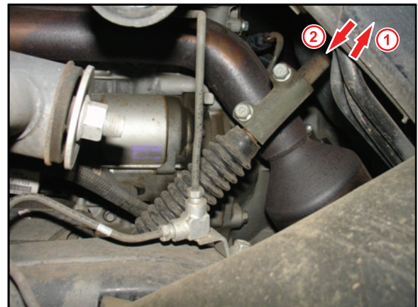
1 Slide Intermediate Shaft Into Column First 2 Slide Intermediate Shaft Into Lower Shaft Second
